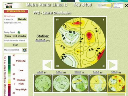
Fig.4 Lateral PFE Distribution View (SCAN mode); Forecast results of a high fracture porosity zone with small cavities (<0.5m ø), high-medium water-inflow
