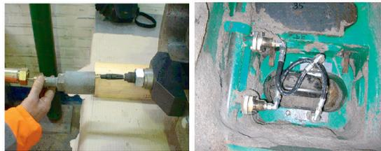
e.g. Connection and protection of isolated A0-contacts ("measuring electrodes")
